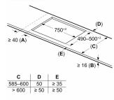
Measurements in mm
