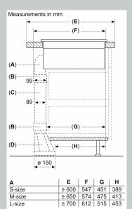
A: 90° Bow B: Connector sleeves C: Straight tube D: Straight adapter round flat
